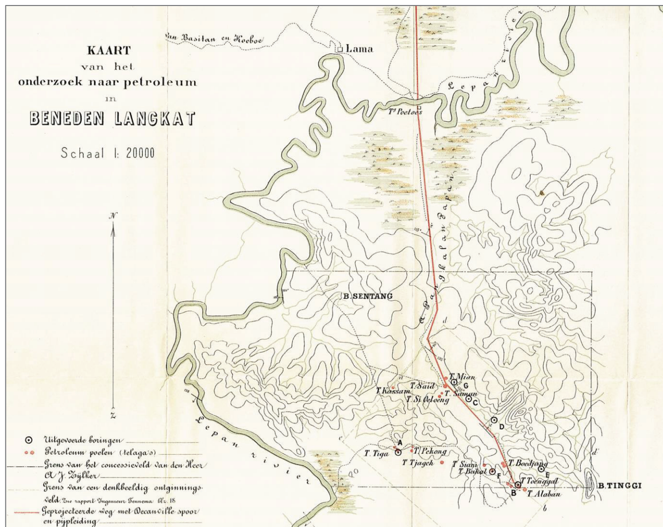
Fig. VI.94. Map of the petroleum survey work and drilling on the concession of A.J. Zijlker, showing locations of 18 oil seeps and 6 shallow wells drilled by Mijnwezen personnel, and a proposed pipeline route in (red line; Fennema, 1890). The drilling work and business plans that Fennema prepared for Zijlker were key to the success of Zijlker's oil exploration, and thus to the birth and survival of the Royal Dutch Petroleum Company.
